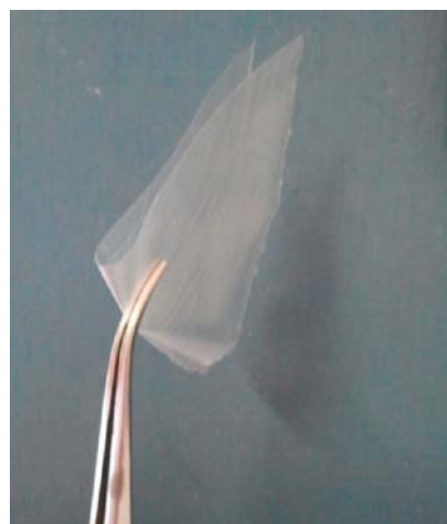
Figure 8. Picture of a starch membrane containing 5 wt % \text{ZP}(\text{C}_6)_{0.54} .
